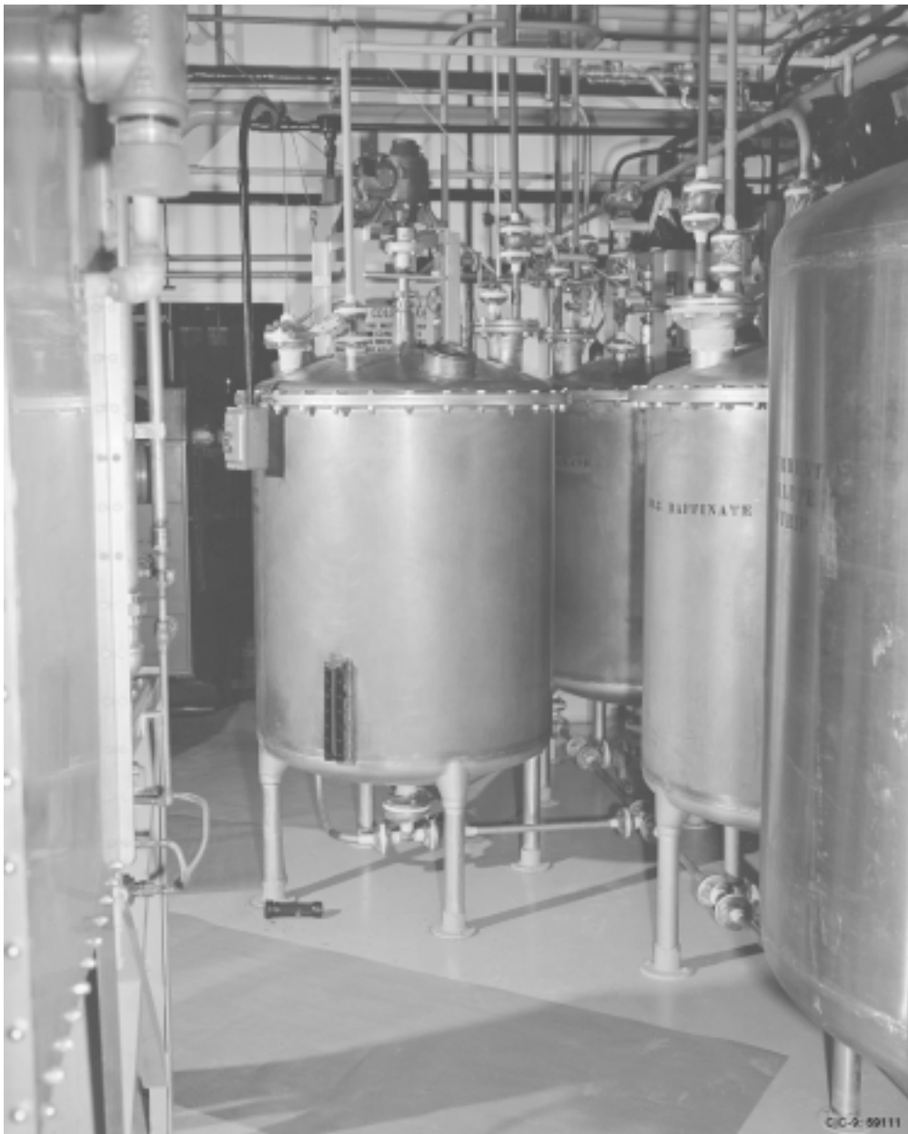
Figure 12. Vessel in which the 1958 Los Alamos process criticality accident occurred.
